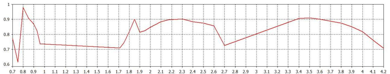
\*Typical efficiency simulated in CST Microwave Studio on 400x400mm (1.3' x1.3') ground plane excluding cable loss
