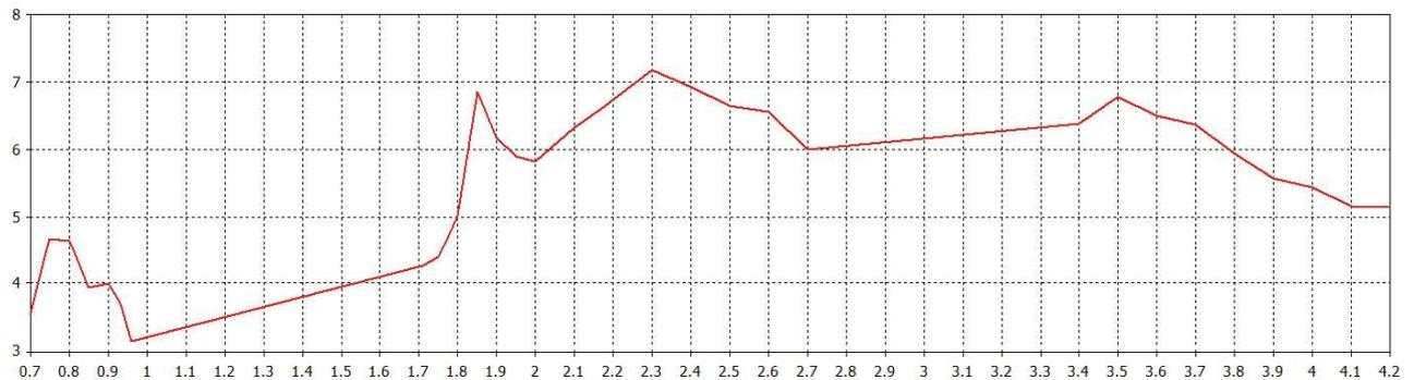
\*Swept peak gain simulated in CST Microwave Studio on 400x400mm (1.3' x1.3') ground plane excluding cable loss
