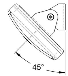
TOP VIEW OF ANTENNA ASSEMBLY SHOWING MAX. ANGULAR POSITION OF 45° (IN BOTH DIRECTIONS). SCALE 1:3
