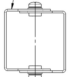
M4 x 6LG. PAN HD. POZI - DRIVE STAINLESS STEEL SCREW IN 2 POSITIONS.
