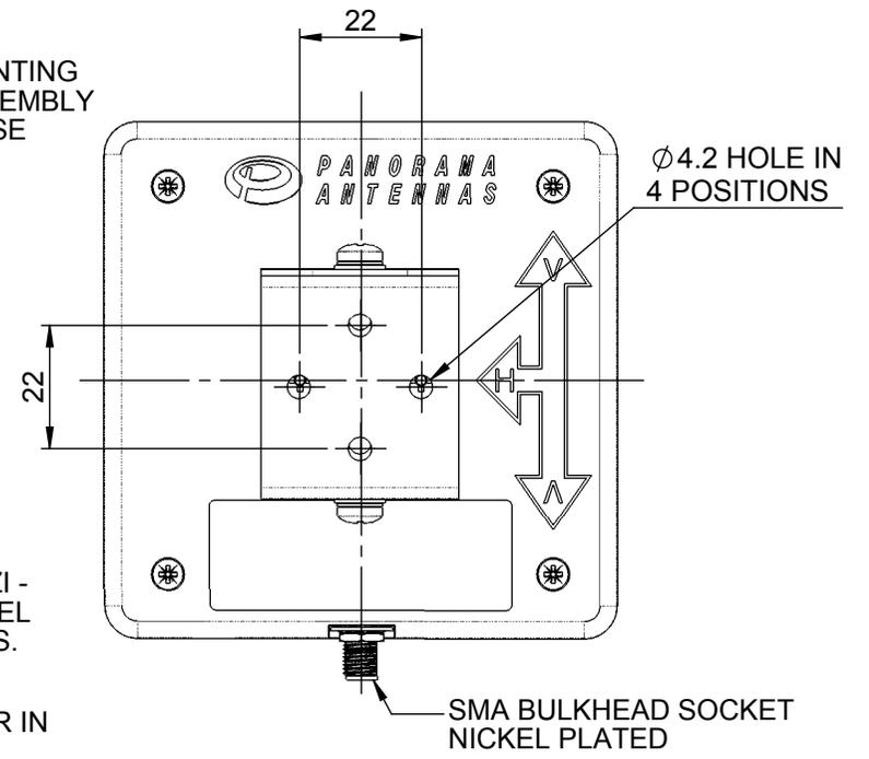
SMA BULKHEAD SOCKET NICKEL PLATED
