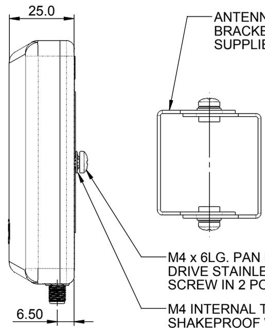
ANTENNA MOUNTING BRACKETS ASSEMBLY SUPPLIED LOOSE
