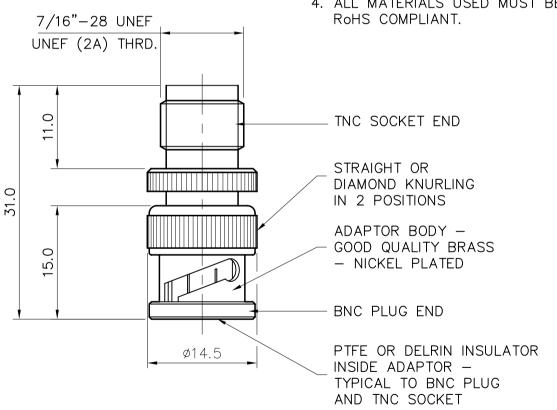
CA-TJ-BP TITLE TNC SOCKET TO **BNC PLUG ADAPTOR** MATERIAL FINISH DRAWN DO.CHECK A.G. SCALE 2:1 DIMENSIONS IN mm TOLERANCES UNLESS OTHERWISE STATED O DEC. PLACE ±0.5 2 DEC. PLACES ±0.1 1 DEC. PLACE ±0.2 ANGULAR DO NOT  $\bigcirc$ PROJECTION SCALE C/NOTE ISSUE DATE 15.07.09 01019
